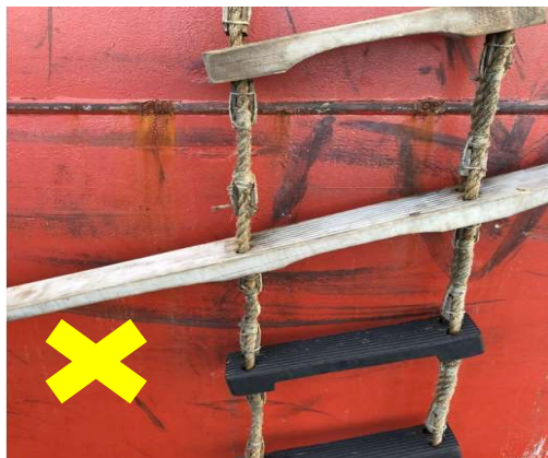
Loose ladder steps & not horizontal
