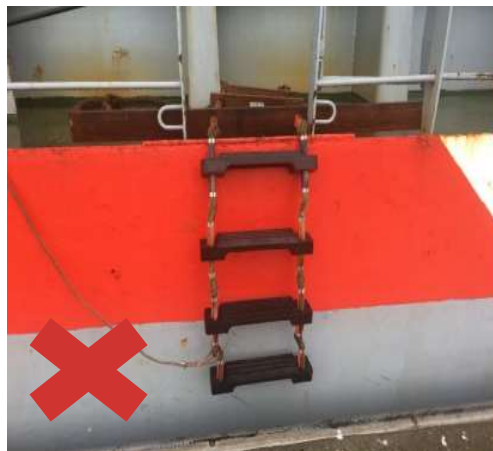
Spreader used for securing
