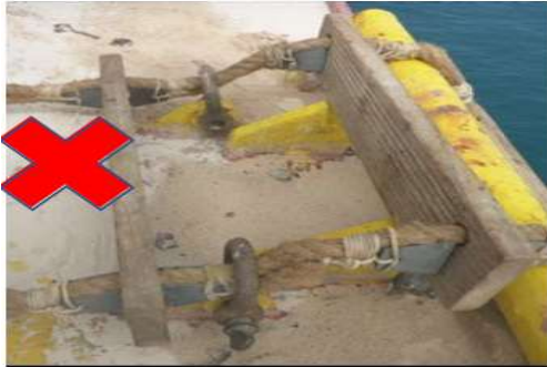
Secured using shackles, risk of damage to the chocks
