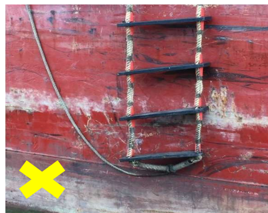
Tripping line incorrectly rigged (must be over the 1 st Spreader from bottom and leading in the forward direction)
