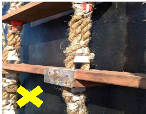
Spreader not made from a single piece of wood
