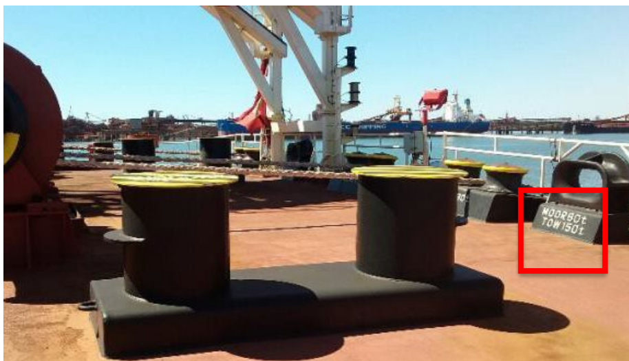
Figure 3: SWL markings on vessel deck fitting
