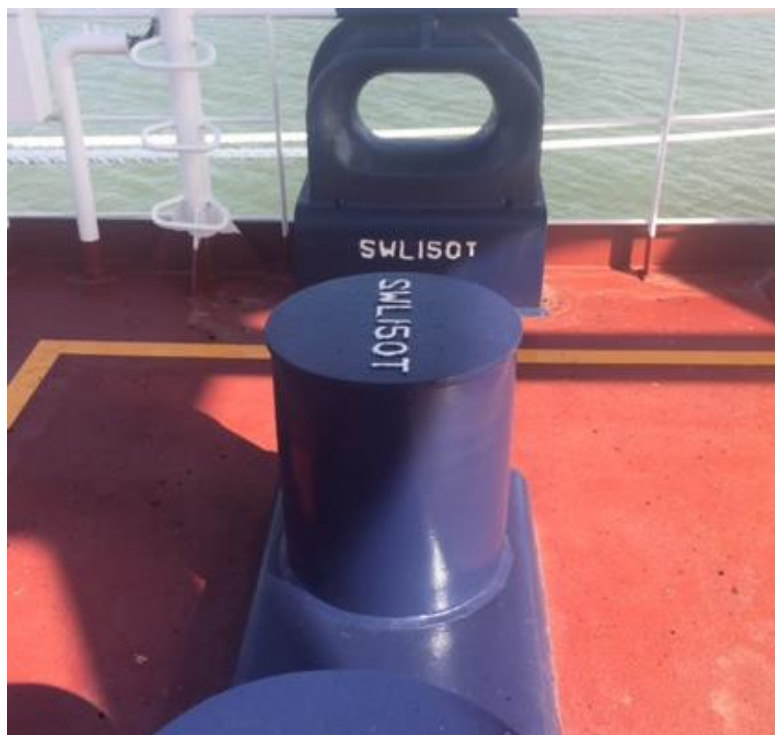
Figure 1: Vessel's bitts and Panama lead on aft deck are suitably aligned and can be used together for towing purposes. Note: the markings in this picture are an example of best practice. PPA requirement is 120T.
