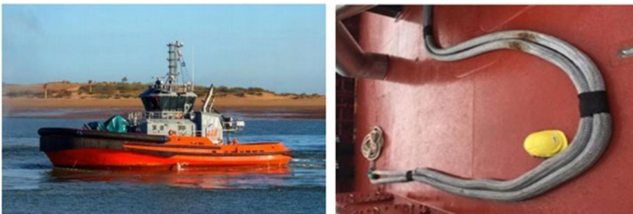
Rastar Tug - 30m of towline grommet = 300kg
