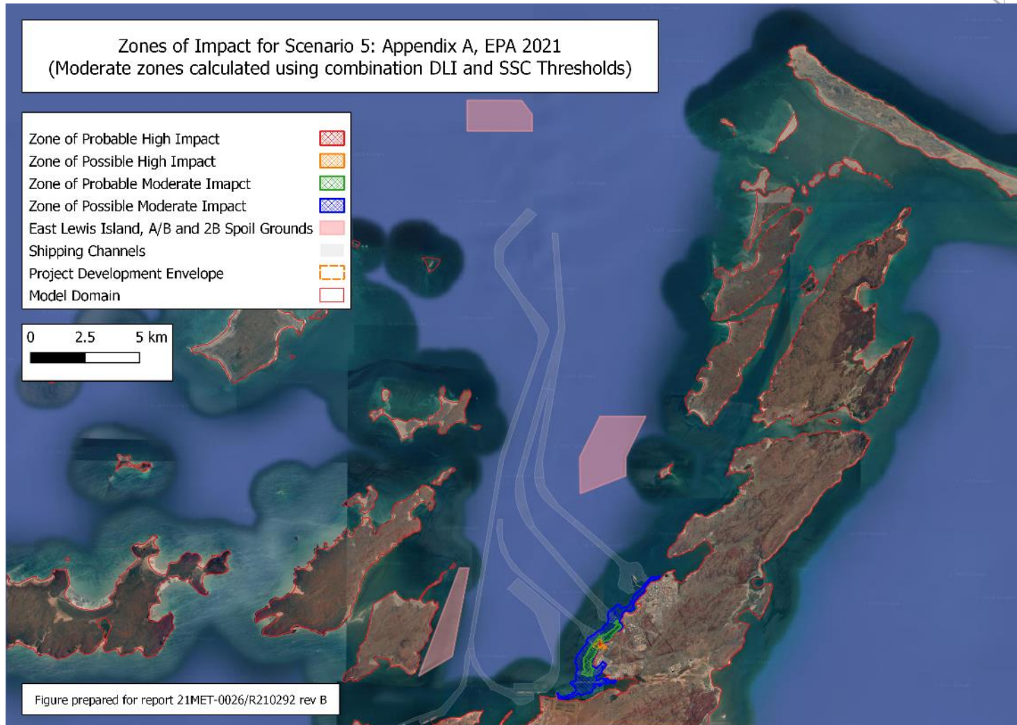
Figure 8 Dredging Zone of Impact showing no ZoMI or ZoHI from disposal at established spoil grounds.
