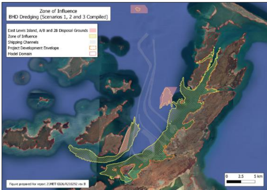
Figure 32 Zone of Influence: Scenario 1, 2 and 3 (Backactor, barge overflow and disposal at East Lewis Island, A/B and 2B).
