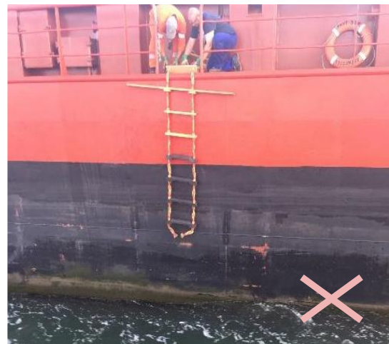
5 th step must be a spreader
