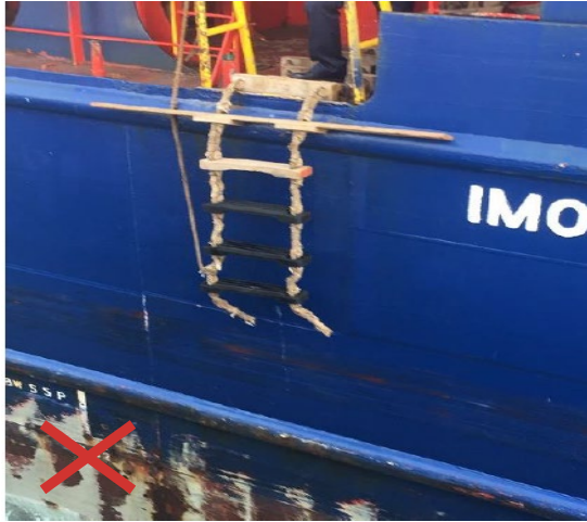
Last four steps must be rubber, incorrect positioning of tripping line
