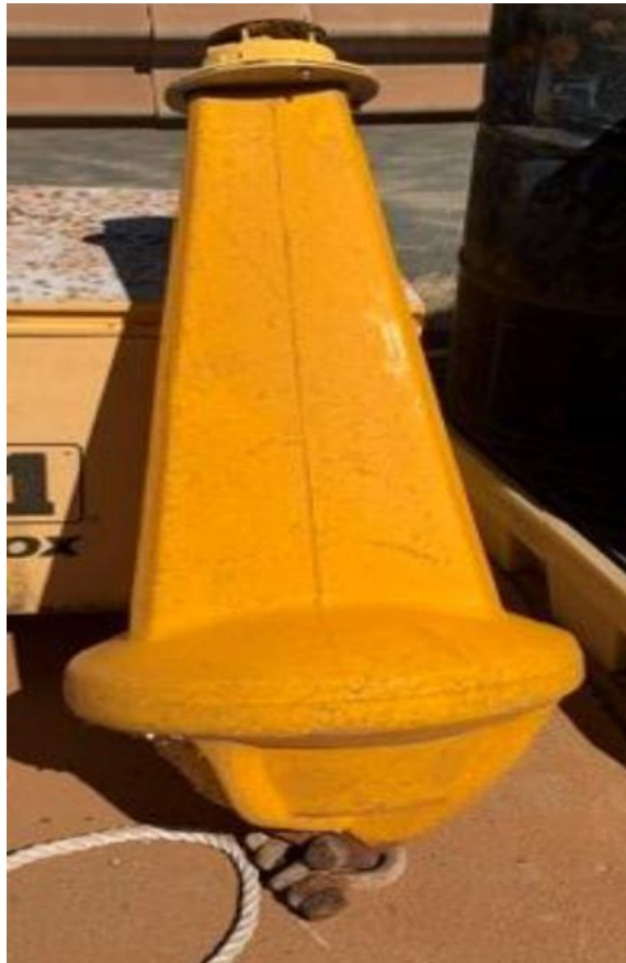
Yellow marker buoy marking the stern anchor of DSV Mary V (FI.Y.1s)
