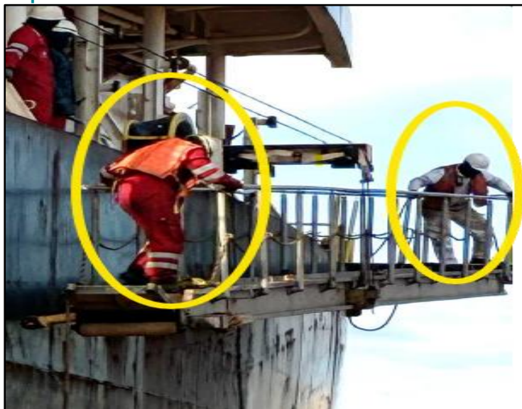
Figure 2: Unsafe accommodation ladder rigging, showing crew working without fall-protection equipment, incorrectly worn PFDs, and support personnel positioned outside ship rails near the ship's side without PFDs
