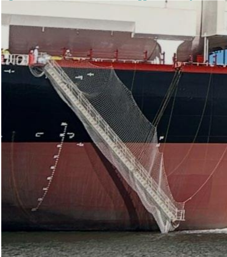
Figure 1: Accommodation ladder rigged correctly
