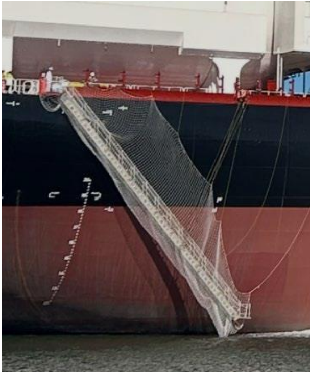
Figure 1: Accommodation ladders rigged correctly
