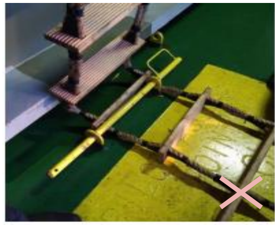
Secured using steel bar, weight on the step
